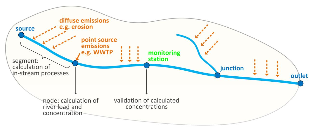
Fig. 1: Schematic concept of the node-and-segment model
